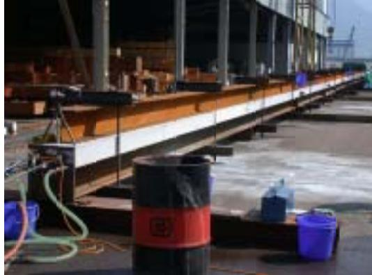
50 m long injection test of the connection
